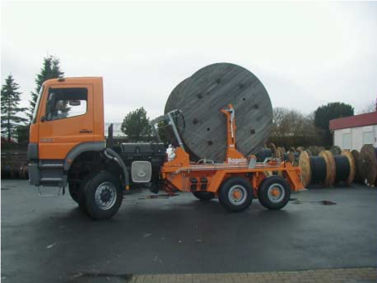
The cable drum trailer BKT 70U is flange-mounted on a Mercedes Atego.
