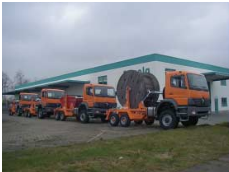
The cable drum trailer BKT 70U is flange-mounted on a Mercedes Atego.
